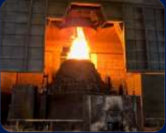
15 ton medium frequency furnace
