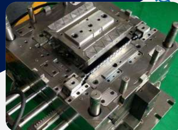
Automotive air conditioning tissue mold Grade: TGE11 working life: 80—100 thousand times
